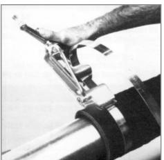
4) When maximum tension has been reached, roll tool over buckle. At same time reversing handle carefully approx. 3/4 turn to avoid breakage. The band that is released will be used in the bend and therefore there is no loss of tension.
