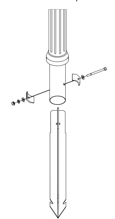
2. Slide post over the star stake until it rests on the stake's notched edge. Using a bolt, (2) washers, (2) extruded washers, a lock washer and nut, attach the pole to the star stake, through the central mounting hole.
