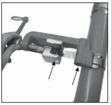
Place band in open of tool nose and gripper block. Move into slot as far as possible to avoid buckle sliding into tool nose. Apply tension by turning handle of tool.
