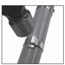
8. Hammer down buckle ears to hold band stub in place to complete clamping.
