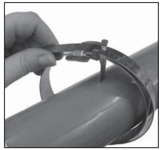
Continue band around object once more and again through buckle. Double banding develops a great deal more radial compression than single banding. Bend end of band under buckle.
