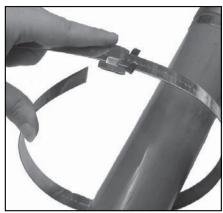
Band may be used from bulk roll as this completely eliminates waste of band. Slide buckle on band as shown, bringing end of band around object to be clamped and again through buckle.
