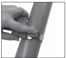
4. Place finger on band at buckle bridge while tensioning with the tool handle. As you are turning handle, maximum pressure is being exerted by the band around object being clamped. Stop turning handle.
